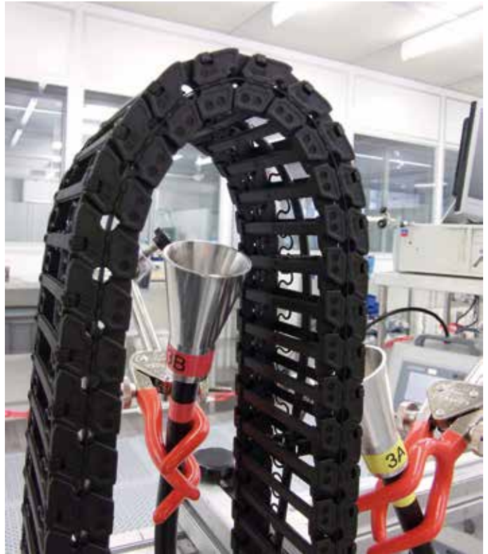
Testing HELUKABEL® CLEANFLEX® cables under cleanroom conditions
