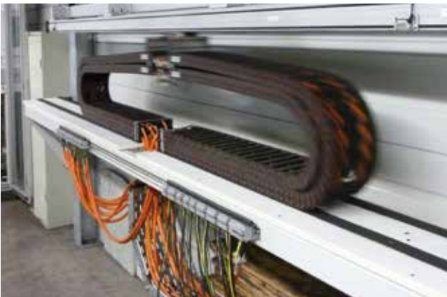
3 m drag chain test facility
