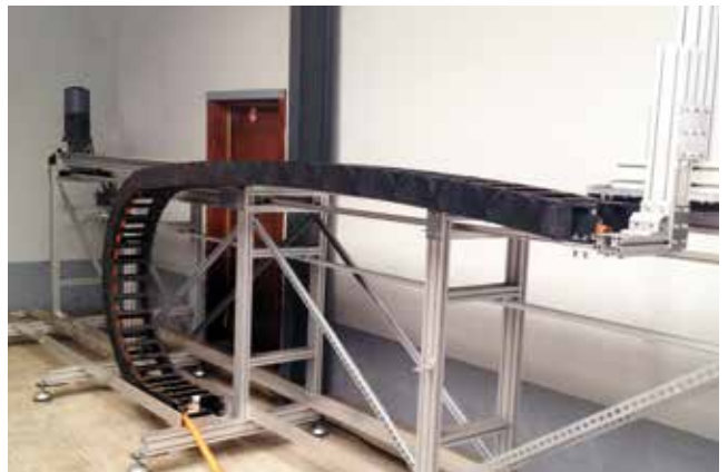
6 m drag chain test facility for larger cross sections
