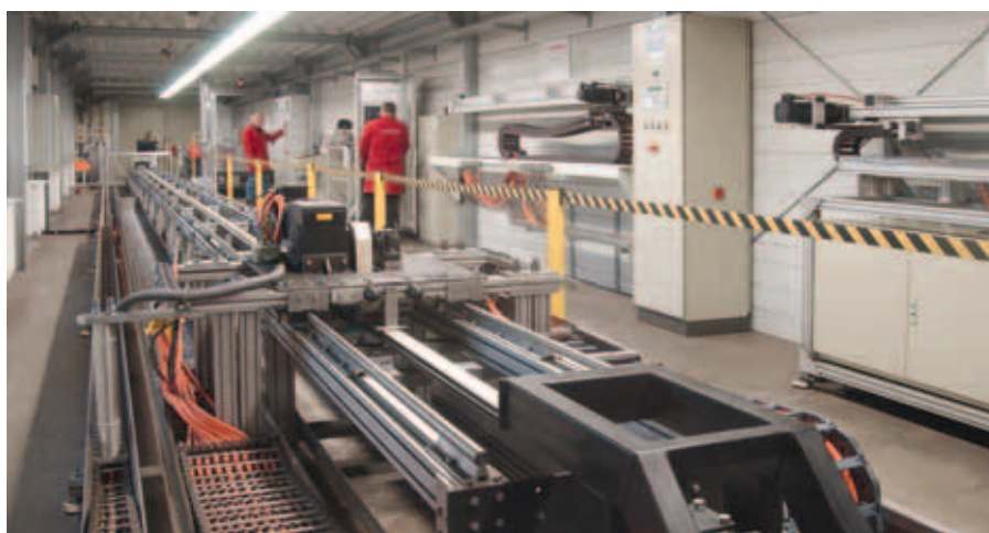
Drag chain test system
