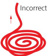
2. The cables must always be attached to the equipment drum without torsion.
