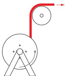
1. The cables are to be pulled from the reeling drum without twisting, using a drawing cable and cable grip. Deflecting or pulling the cable over edges should be avoided.
