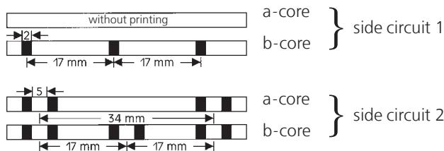
The cores of 5 star quads of a sub unit are counted according to the sequence of basic colours:
