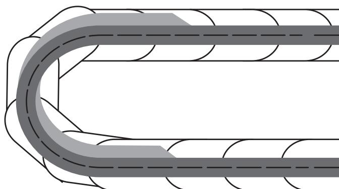
2. The cables must be installed with guide stays, dividers or in separate hole stays so as to move freely in the drag tray guides. As free space for the cables in the guide stay should be at least 10% of the cable Ø.
