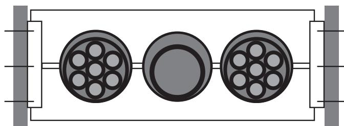
1. Where flat and round cables are mixed in one drag tray, then these should be installed loosely next to one another. The guide stays should be installed between the cables laid side by side. Try and avoid placing different sizes of round cables next to one another. Due to the limited space relationship cables arranged one above the other, frame stays are to be installed.
