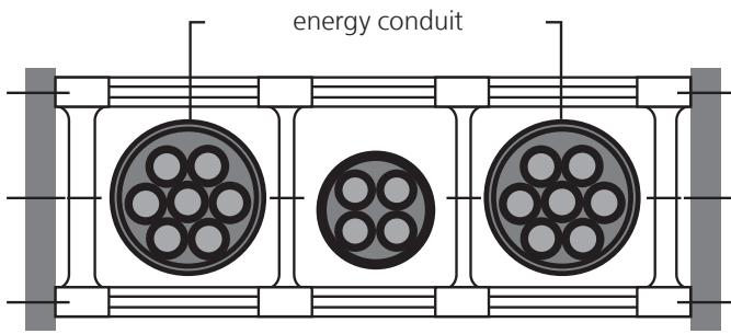
6. In case that is not possible to lay the cables as described under 4, in order to lay several multi core high flexible cables with an outer diameter < 10 mm, we recommend the use of a guiding tube, in which these cables should loosely laied. This tube is than integrated into the drag system. The cross section of this tube has to be much larger as the sum of the cross sections of the cables. For the free movement of the flexible energy conduits, the guide or divider stays must be installed.
