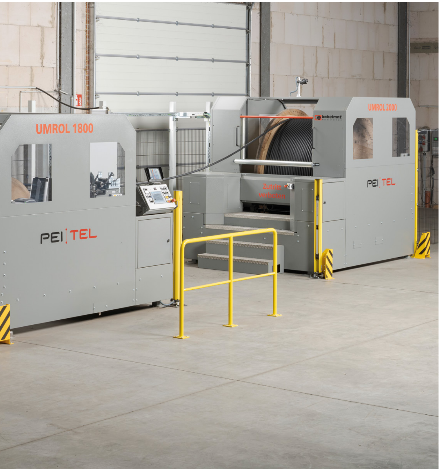
A KABELMAT automatic rewinding line makes the protective handling of delicate cables at pei tel possible.
