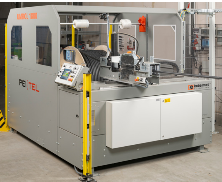
pei tel utilises an UMROL 1800 and an UMROL 2000 to wind and unwind cables.
