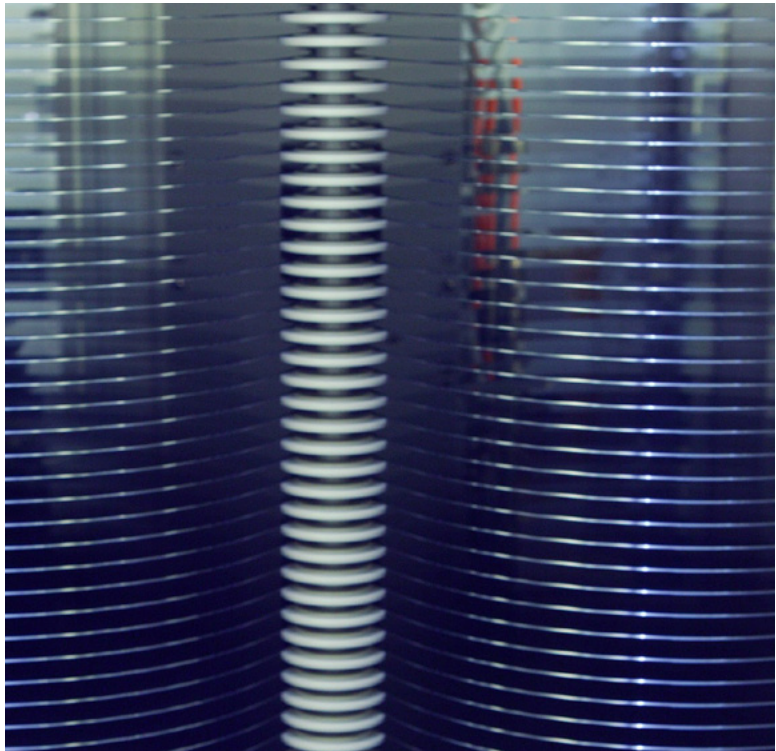
Wafers are round or rectangular sheets of silicon that are less than a millimeter thick. They are the basis for microchips.
