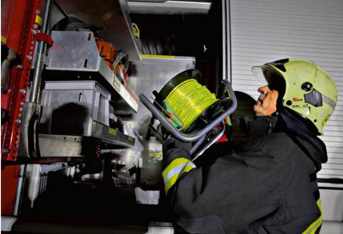
Fire engines are normally fitted with one to three cable drums.
