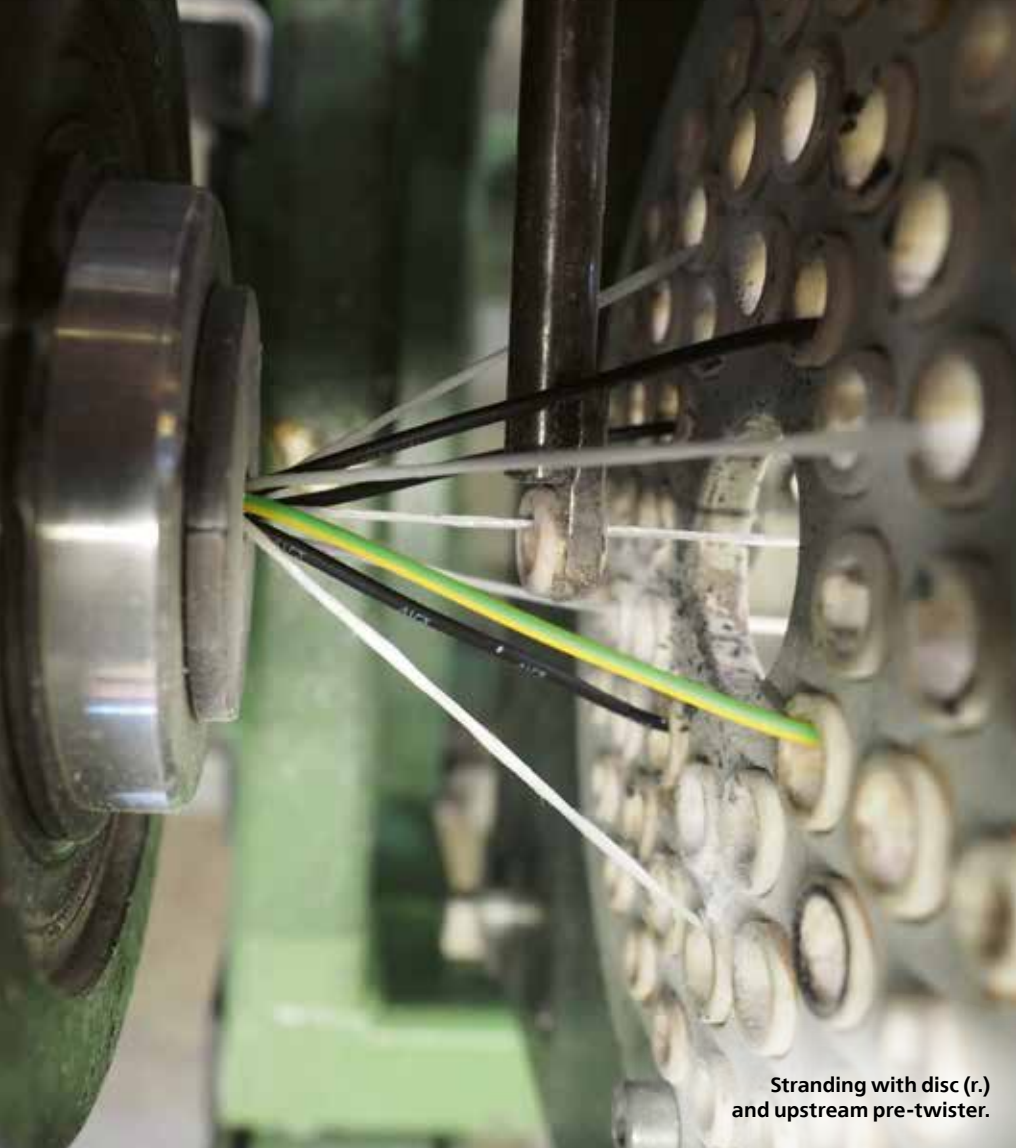
Layers stranded in opposite directions on a planetary machine.
