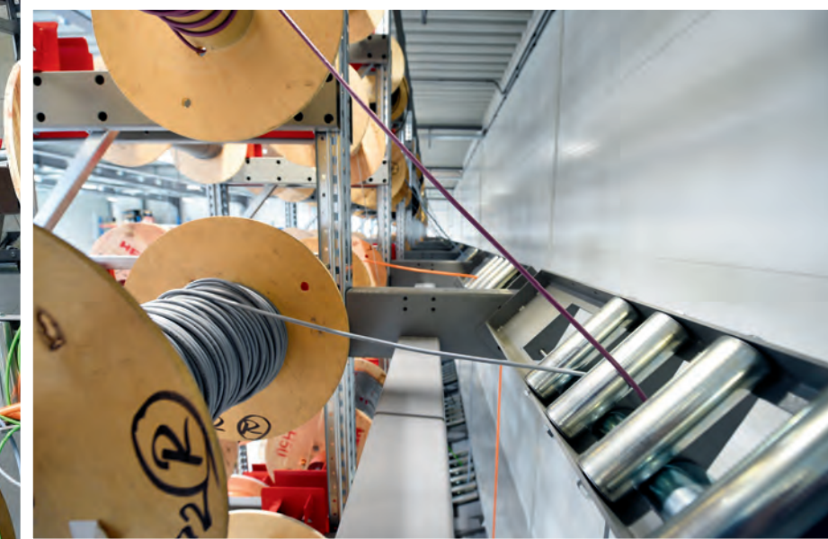
The operator lowers each cable using a pulley, which prevents unused cables from getting in the way when cuts are made.
