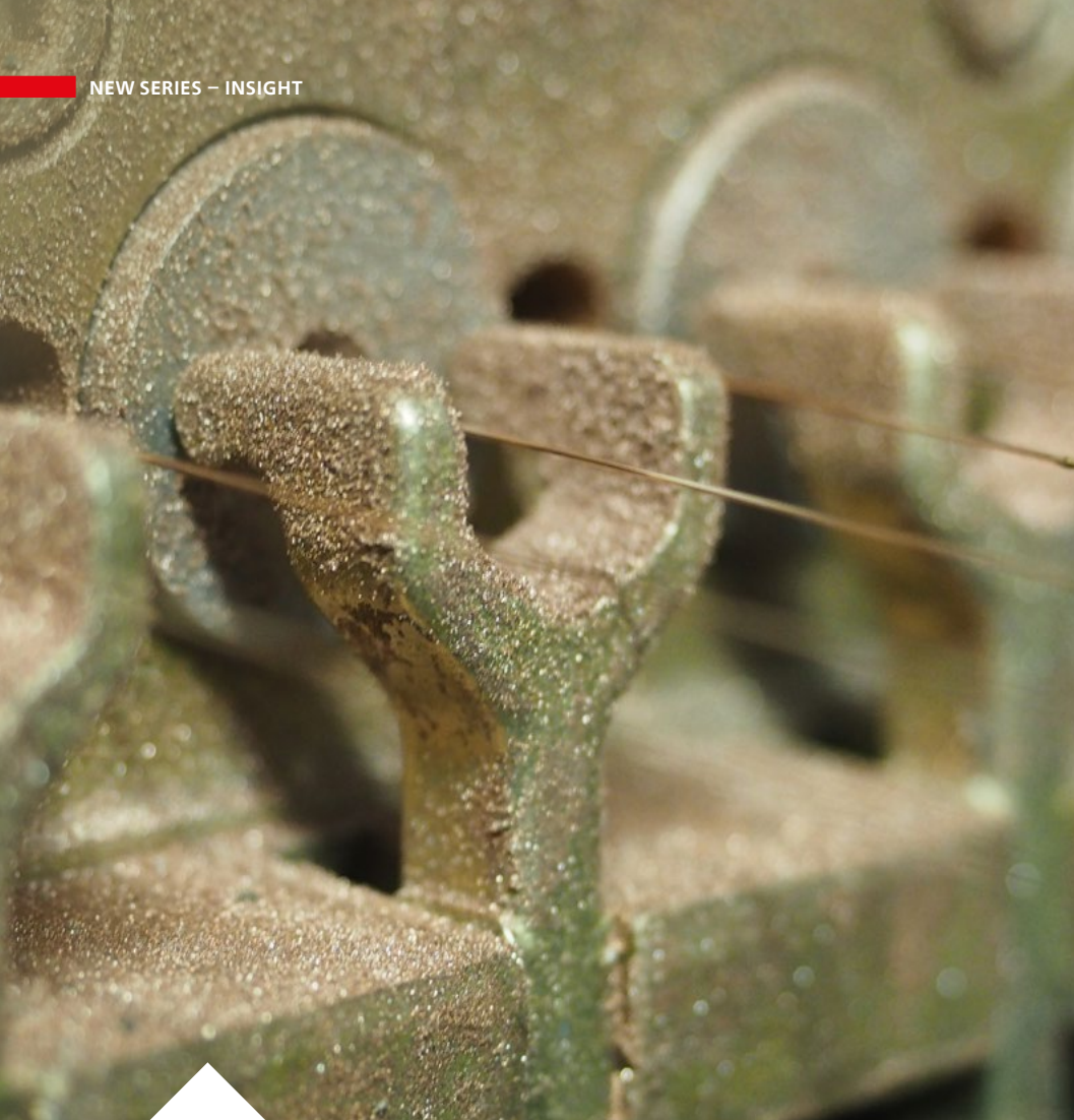
The emulsion is used for cooling and lubrication while also stopping the wire from oxidising.
